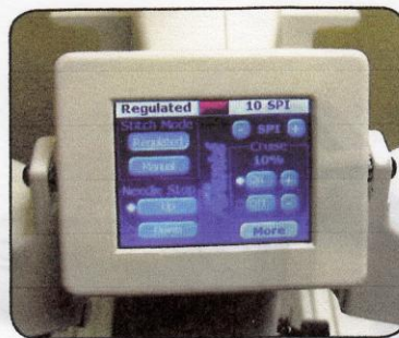
COLOR TOUCH-SCREEN ON FRONT AND BACK HANDLEBARS
